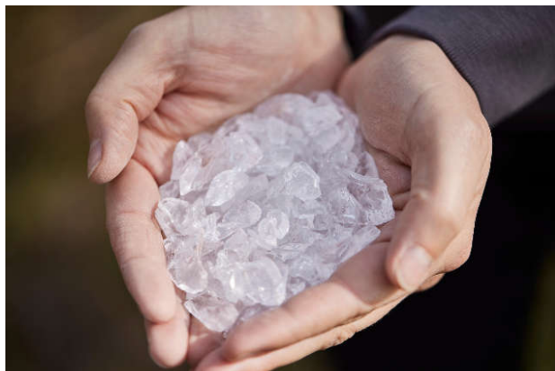
Production scraps from fiberoptic cables containing germanium
